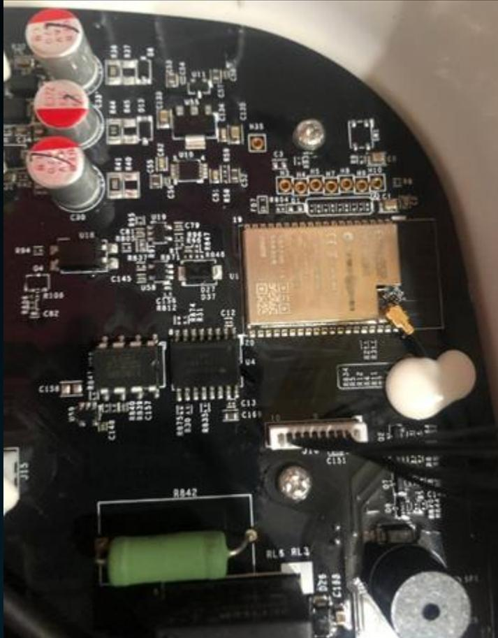
ESP32 Microcontroller with exposed serial interfaces
