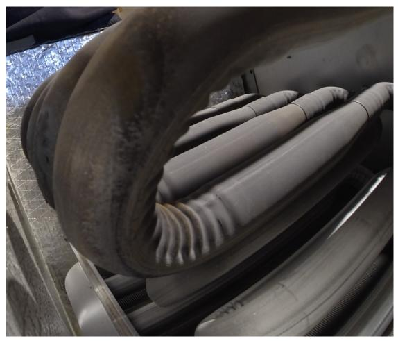
Heat exchanger fails/cracks
